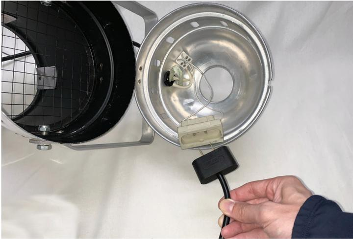
GX16D Socket Power Connection Complete
